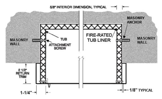
INSTALL SCREWS THROUGH BOTH TUBS INTO MASONRY ANCHORS Fasten cabinet with a minimum of 4 screws per cabinet
