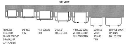
\*Note: For surface mount cabinets, add 3 3/16" to width and height measurements. See product page for wall opening dimensions.
