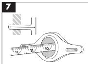
**DETERMINE THE DRAIN NIPPLE DEPTH**
