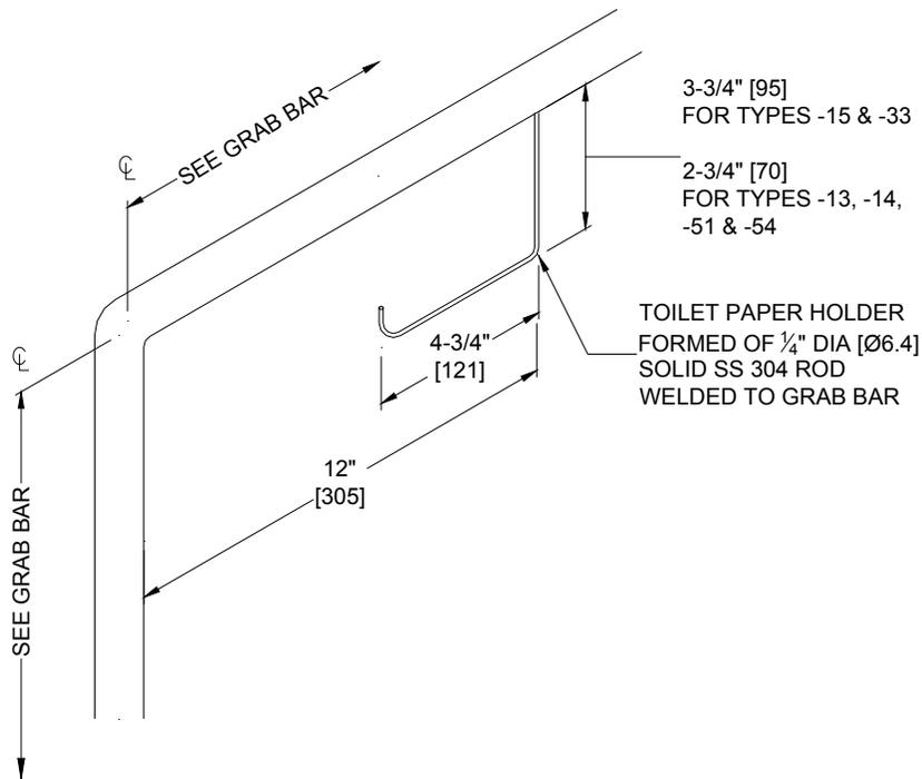
Option -25 Toilet Paper Holder is welded on to Grab Bars of the Swing Up or Swing Away configurations 3413, 3451, 3454 and Fixed Types -15, -33
