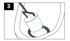
Lift and tilt cartridge to drain all free liquids then spray Falcon Foam Cleaner into housing.
