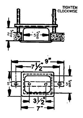
ANCHORING METHOD FOR WALLS OVER 2-3/4" THICK
