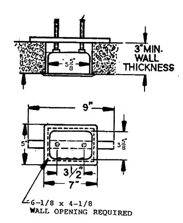
DIRECTIONS: Models for wall thickness up to 2-3/4 thick are furnished with a rustproofed steel bolted back plate. The back plate has two 1/2" rustproofed adjusting studs, which when turned clockwise, pull the rim snugly to the wall, permanently anchoring the assembly. Models for thicker walls are similar except the back plate is furnished with 1/4" full thread rustproofed studs and nuts which permanently anchor the assembly.
