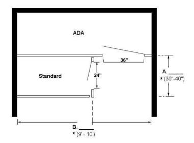
\*Dimensions shown are for a common bathroom stall size. In most cases stalls can be made to fit any size or configuration.
