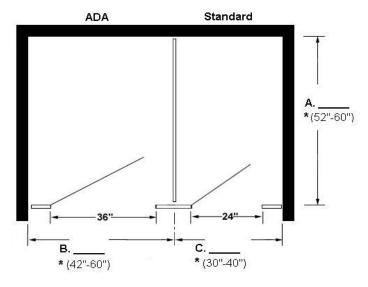
\*Dimensions shown are for a common bathroom stall size. In most cases stalls can be made to fit any size or configuration.
