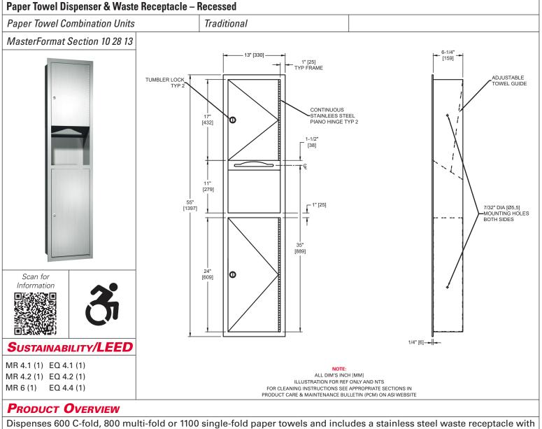
the capacity of 7 gal. (26 L). Adjustable guide provided to allow dispensing of multi-fold or C-fold paper towels.
