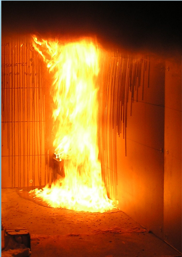
Standard NFPA 286 test method with HDPE untreated panels mounted on fire test room walls.
