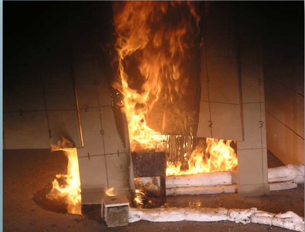
HDPE untreated panels being tested as they would be installed as toilet partitions in the field.
