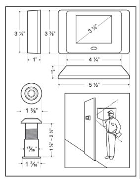
The Electronic Digital Door Viewer (ELECDDV180) is an innovative product designed to replace conventional peephole door viewers with an electronic video system that delivers on-demand and high quality images. This avoids caller from the outside to see any movement from the inside when they come knocking. Unwanted callers can be ignored or screened without them knowing there are people inside. Ensures your privacy is protected.
